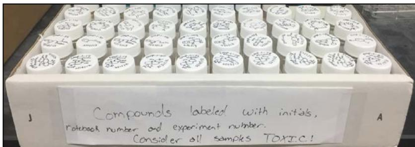
**Figure 3:** Research samples labeled with initials, notebook number are contained within a holder labeled with the hazards
